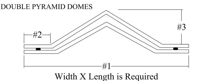
The above shape is the only option available. If there is a 90 degree bend where the flange (dim #2) intersects the dome rise, our replacement domes will not fit your frame. It is the purchasers responsibility to confirm shape and compatibility with the existing frame.
