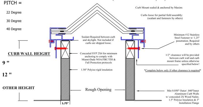
\*\*Meets OSHA Fall Protection guidelines with no additional coverage/screen required OSHA 29 CFR 1910.23 & 1926.501 Fall Protection Required for Roof Openings
