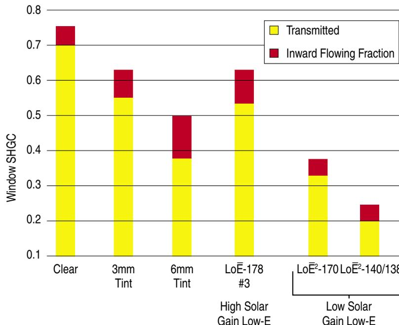
Window SHGC is the summation of heat gains through the transparent and opaque areas. Frame area is the biggest variable affecting the opaque region. The magnitude of solar gains through the frame is minor - typically less than 2% impact on the window SHGC.
