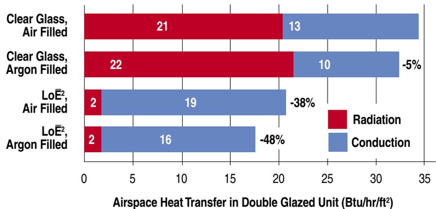
Figure RB15-3 shows how glass performance can be expanded far beyond the basic number of layers through the inclusion of low-E and argon. The heat loss through ordinary double glazing will be cut in half and triple glass unit can perform like 8 panes.
