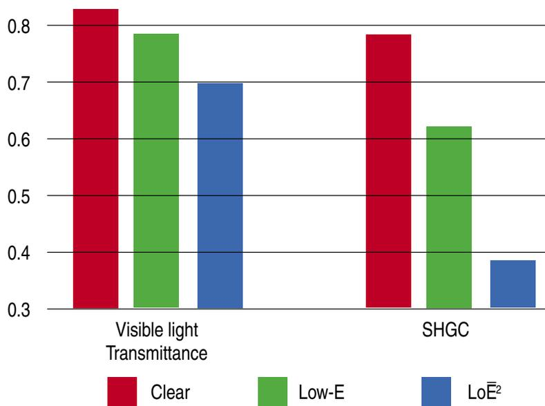
**Fig. RB19-3 Comparison of Insulating Value and Solar Gain**
