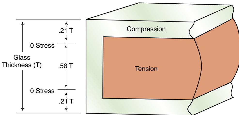
Tempering is a process where annealed float glass is heated to near its softening point (approximately 1300°F) and then rapidly cooled with air. The resulting compression layer increases the glass strength to nearly 4 times that of ordinary annealed glass.
